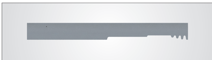
Aerodynamic optimized blade profile
